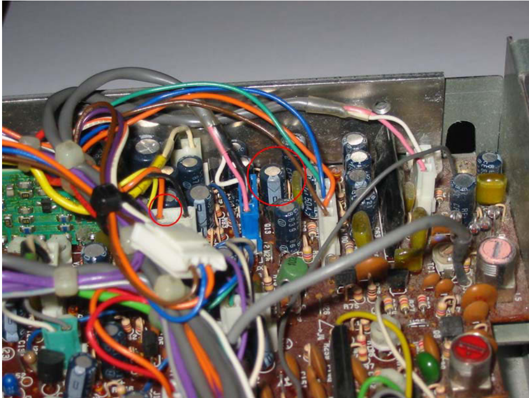
Photo 2: The corner of the board "IF Unit" seen when the upper case is removed. You can see the C69 capacitor at the rear, behind C76, between the 2 connectors J2 (blue) and J6 (white), close to board edge. You can also see the J3 connector (white) with its orange wire connected to the +8V.
