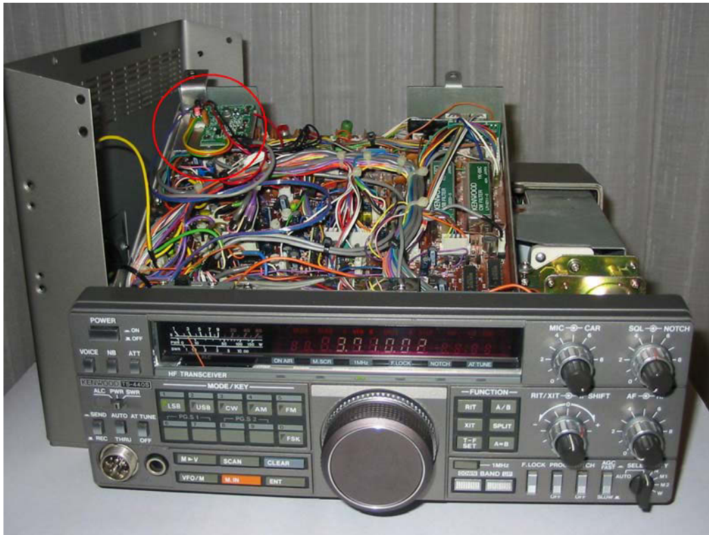
Photo 5: The TS440 in modification. You can see the DSP module installed in top on the left of the "IF Unit" board which was raised.
