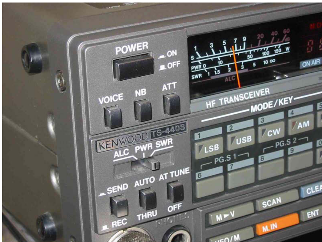
Photo 6: In the left higher angle of the TS440 front, near to the PB "Power" you find the PB "Voice". If option VS1 (Voice Synthetizer) is not inside, this push-button is available to control the DSP.
