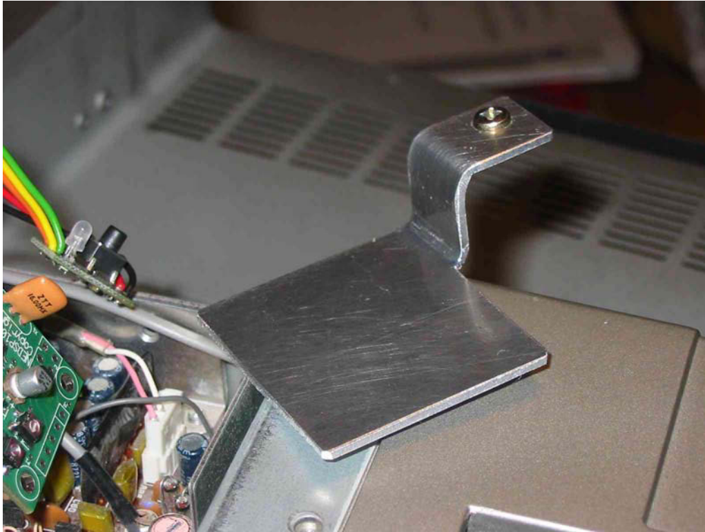
Photo 3: Manufacturing of the support to fix the DSP module. The flat part approximately measures 40 mm x 40 mm.
