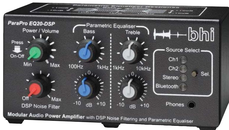
1 kHz to boost or cut. The grey knob at top right is the **TREBLE** tone control, which boosts or cuts the frequency from 1 kHz to 10 kHz. At bottom left, the red knob is the **DSP NOISE FILTER** control. It ranges from **OFF** (bypassed) to **MAX**. At bottom center, the second blue knob is the **BASS** boost/cut control, allowing the selected frequency to be boosted or cut by -10 to +10 dB. At bottom right, the grey knob is the **TREBLE** boost/cut control, again -10 to +10 dB.
