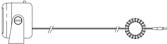
Figure 8. Power lead suppression with ferrite fitted
