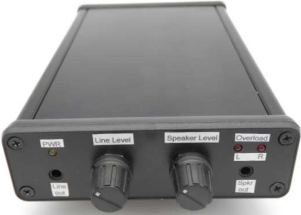
Front Panel of PCB fitted to Hammond manufacturing 1455L1602 case
