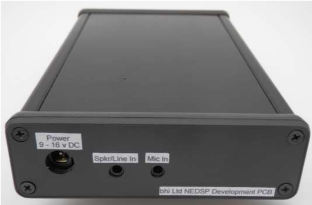
Rear Panel of PCB fitted to Hammond case
