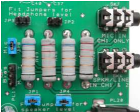
Above: Jumpers set for Speaker Level Inputs
